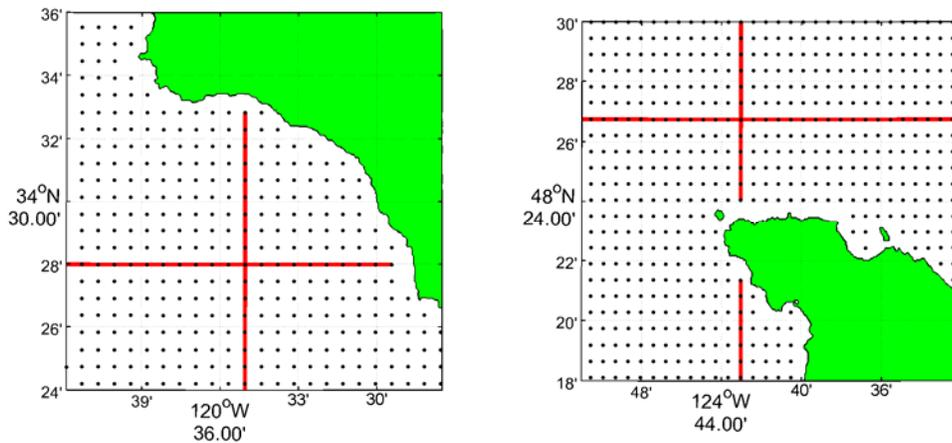
**Figure 3.** Images of the same region show in Figure 1 for the US West coast grid based on an equidistant cylindrical projection. Vertical resolution is constant throughout the grid at 1 km while horizontal resolution increases from 1 km at the southernmost latitude ( $30.25^{\circ}$  N) to 0.75 km at the northernmost latitude ( $50^{\circ}$  N). Arbitrary grid lines highlighted in red show orthogonality is preserved throughout the grid.
