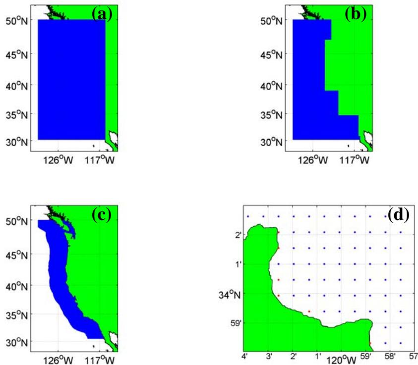
**Figure 1.** The Equidistant cylindrical grid blank for the U.S. West Coast is shown in panel (a). The same grid, after initial gross point elimination is shown in panel (b). Panel (c) shows the grid after points falling over land and outside of the 300km boundary have been removed. Grid points shown in red in panel (d) indicate points that were eliminated from the northeast region of Santa Rosa Island due to their close proximity to land (within 0.5 km).
