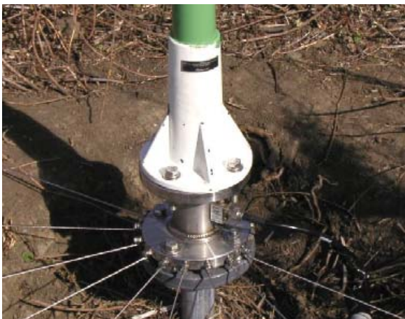
Figure A8. CODAR Long-Range Transmit antenna mounted to the 3" schedule-80 PVC flange.
