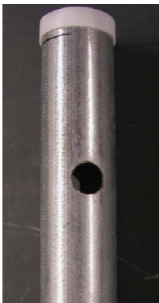
Figure A3. 1" hole required to insert rebar for twisting the screw anchor into the ground.
