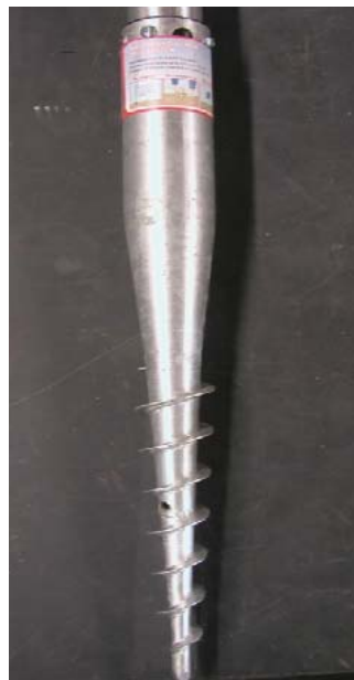
Figure A4. Showing two of the four #14 × 2" sheet metal screws that connect the auger to the EMT.
